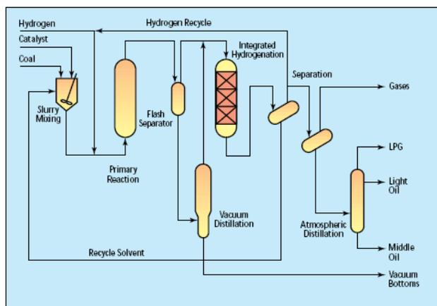
dissolution of a high proportion of coal in a solvent at elevated temperature and pressure, followed by the hydro cracking of the dissolved coal with H<sub>2</sub> and a catalyst. Direct liquefaction is the most efficient route currently available. Liquid yields in excess of 70% by weight of the
