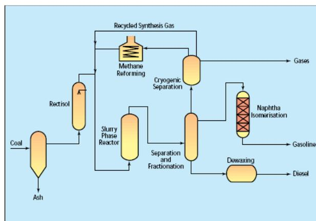
sulphur containing catalyst poisons. The resulting 'synthesis gas' is reacted over a catalyst at relatively low pressure and temperature. The products may be paraffins, olefinic hydrocarbons or alcohols (particularly methanol), depending on the catalyst selected and the reaction conditions used.
